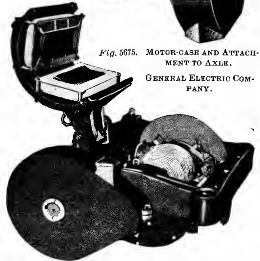
Fig. 5677. MOTOR-CASE AND ATTACHMENT TO AXLE.
